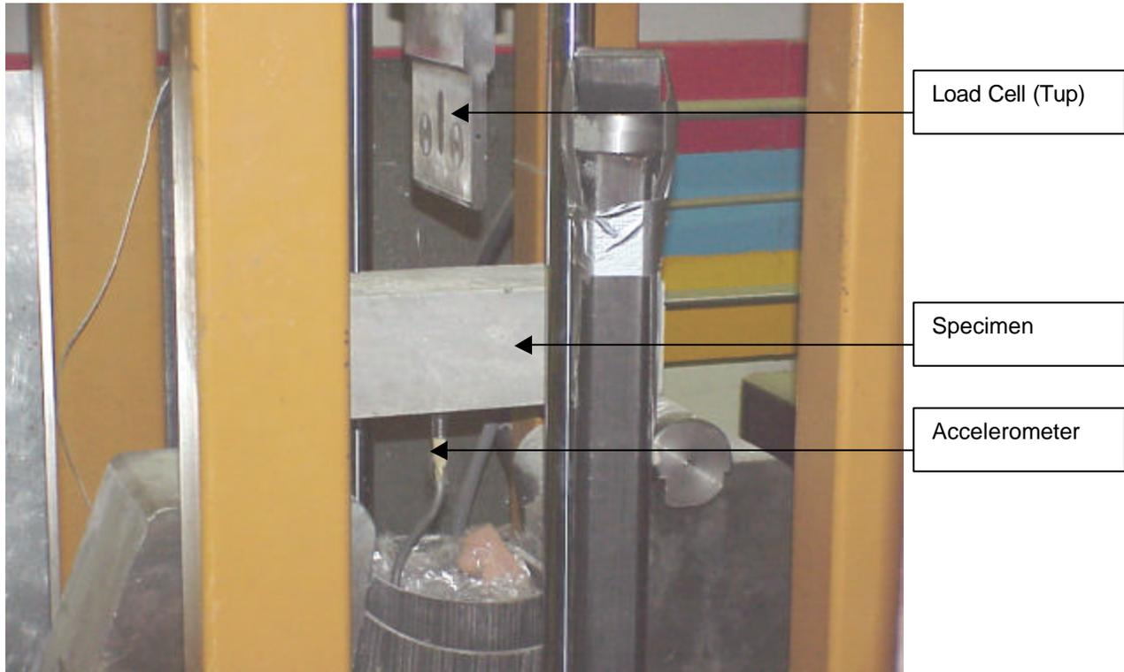
Four drop-heights (200 mm, 500 mm, 750 mm and 1000 mm) were investigated to help describe the impact behaviour under a range of stress rates.
