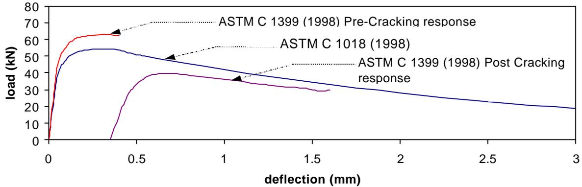
ASTM C 1399 test is recommended for low modulus-low volume fraction fiber reinforced mixes. CRC, with its very high steel fiber content is clearly suited for tests with the ASTM C 1018 or the JSCE SF 4 methods, given that it is practically impossible to replace the steel plate upon first crack (as is required by the ASTM C 1399 method). Consequently, considerable damage occurs to the beam prior to the reloading.
