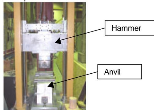
Figure 3. Instrumented Striker ('tup')
