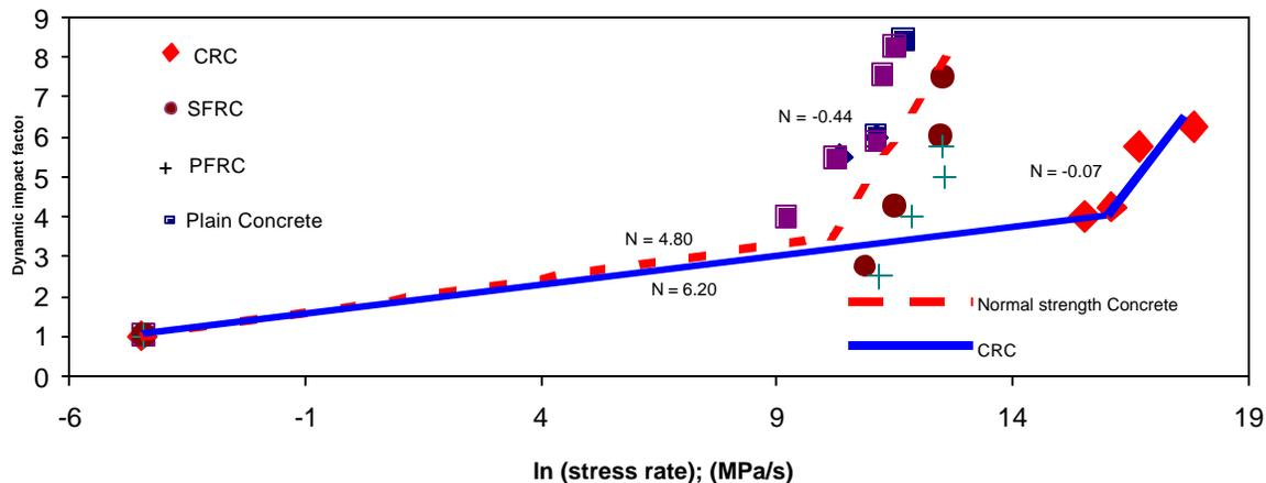
The impact behaviour of CRC highlights several interesting features. As expected from high strength concrete, CRC exhibits a less sensitive behaviour to high stress rate. However, because of its high strength and high fiber content, the material is capable of dissipating greater amounts of energy up to very large stress rates as witnessed in Figure 9. Normal strength SFRC and PFRC (polymeric fiber reinforced
