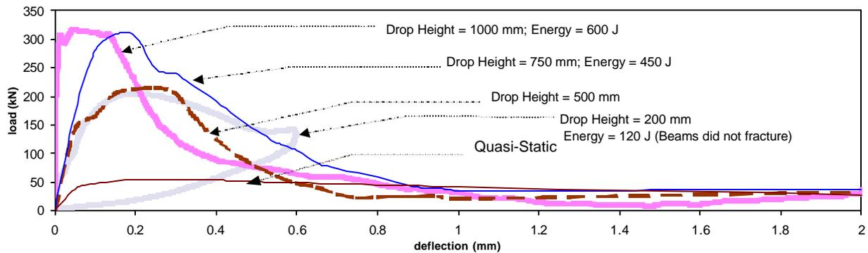
Table 3. Flexural response of CRC under impact loading
