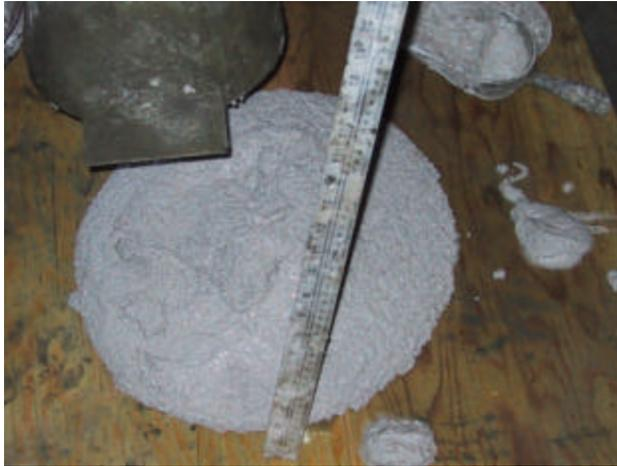
Figure 5. Slump test on CRC mix with 6% fiber
